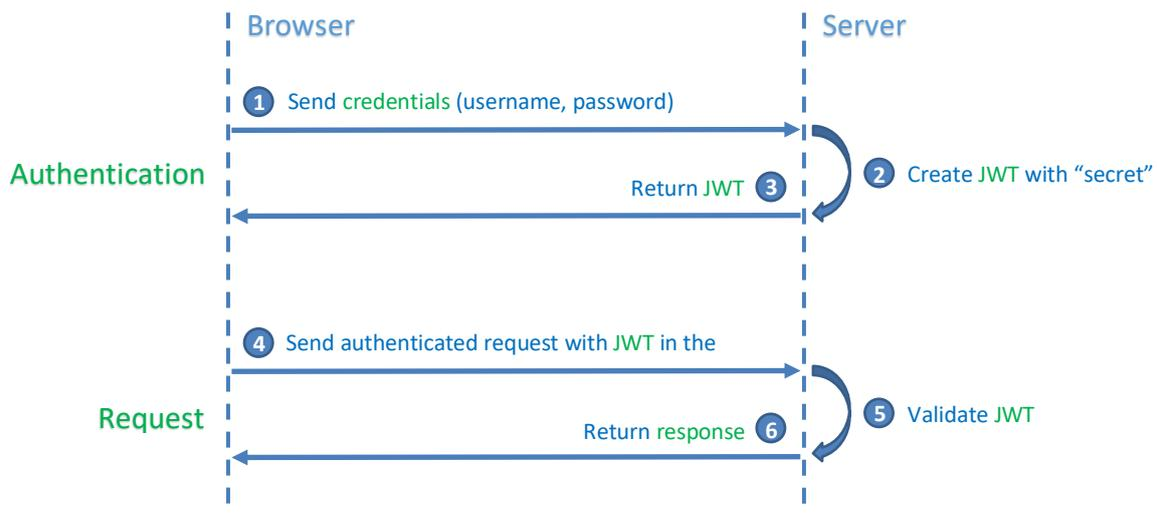
Figure 3: Securely transmitting information between parties with JWT.
